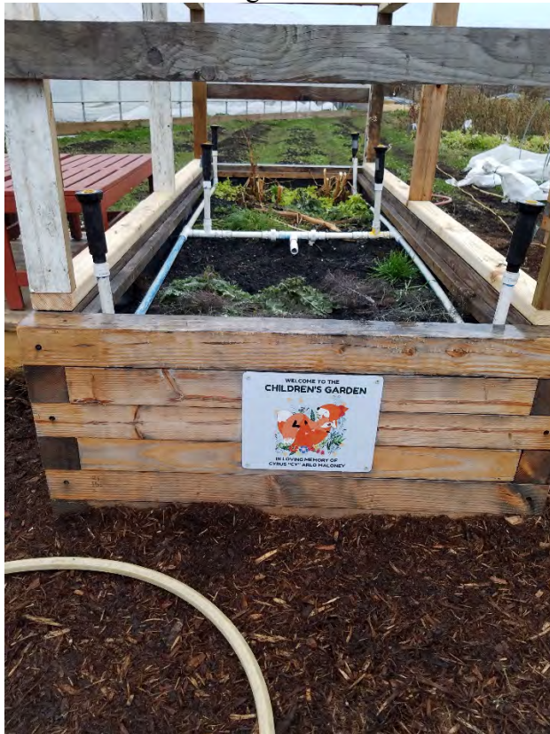
Figure 5: Rainfall Simulator on KGD Raised Beds (Left – prior to wind shield deployment; Right – during simulation)
