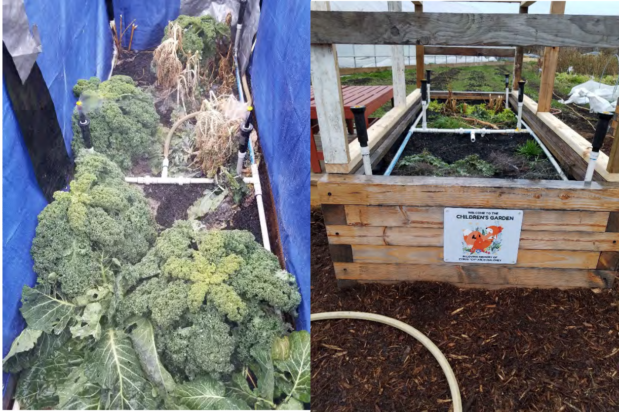
Figure 11: KGD Planting Bed with Rainfall Simulator
