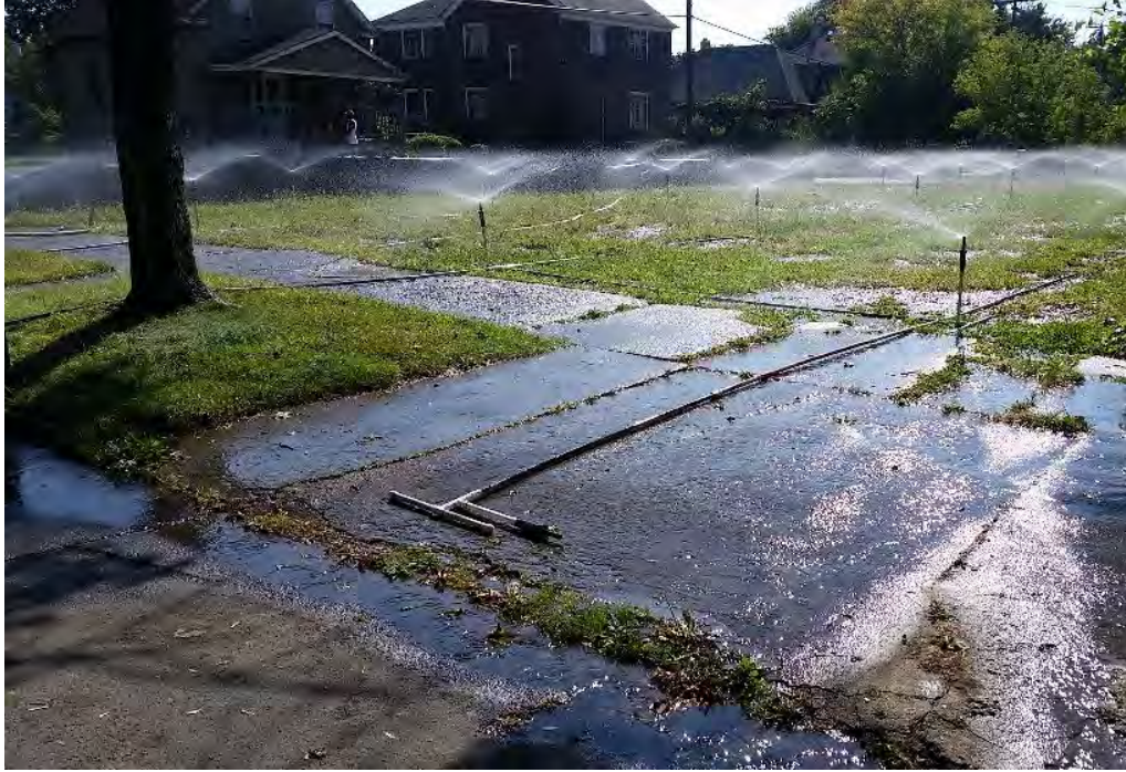
Figure 4: Rainfall Simulator in Use on Vacant Land (2017)
